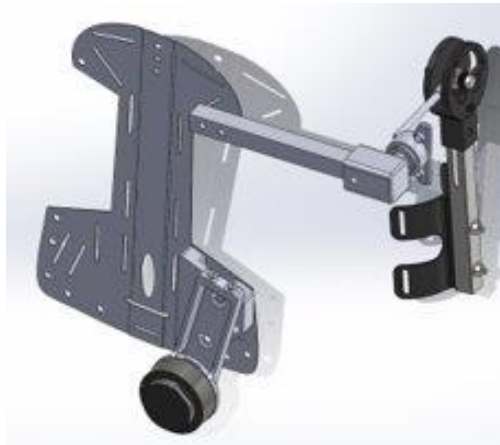
Figure 39: Carbon Fiber Square-Stock instead of All thread
