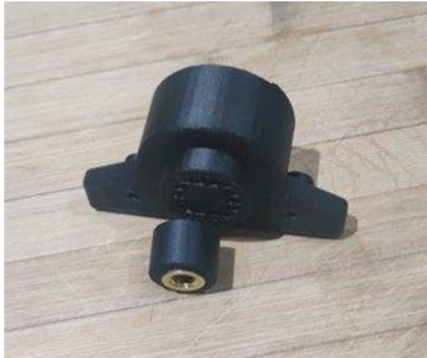
Figure 42: Bowden Cable Termination Block Failure
